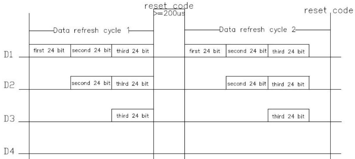
Note: the D1 sends data for MCU, D2, D3, D4 for data forwarding automatic shaping cascade circuit.
